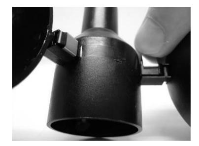
5. Install the Wind Vane Fin Insert the fin into the open end of the wind vane pointer as shown. Press in firmly until a "snap" is felt.
